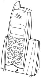
The battery is being charged when the lower green LED on the charger is on (and the battery meter on the display flashes). If the battery is completely flat it can take a few minutes before the lower green LED on the charger comes on.
